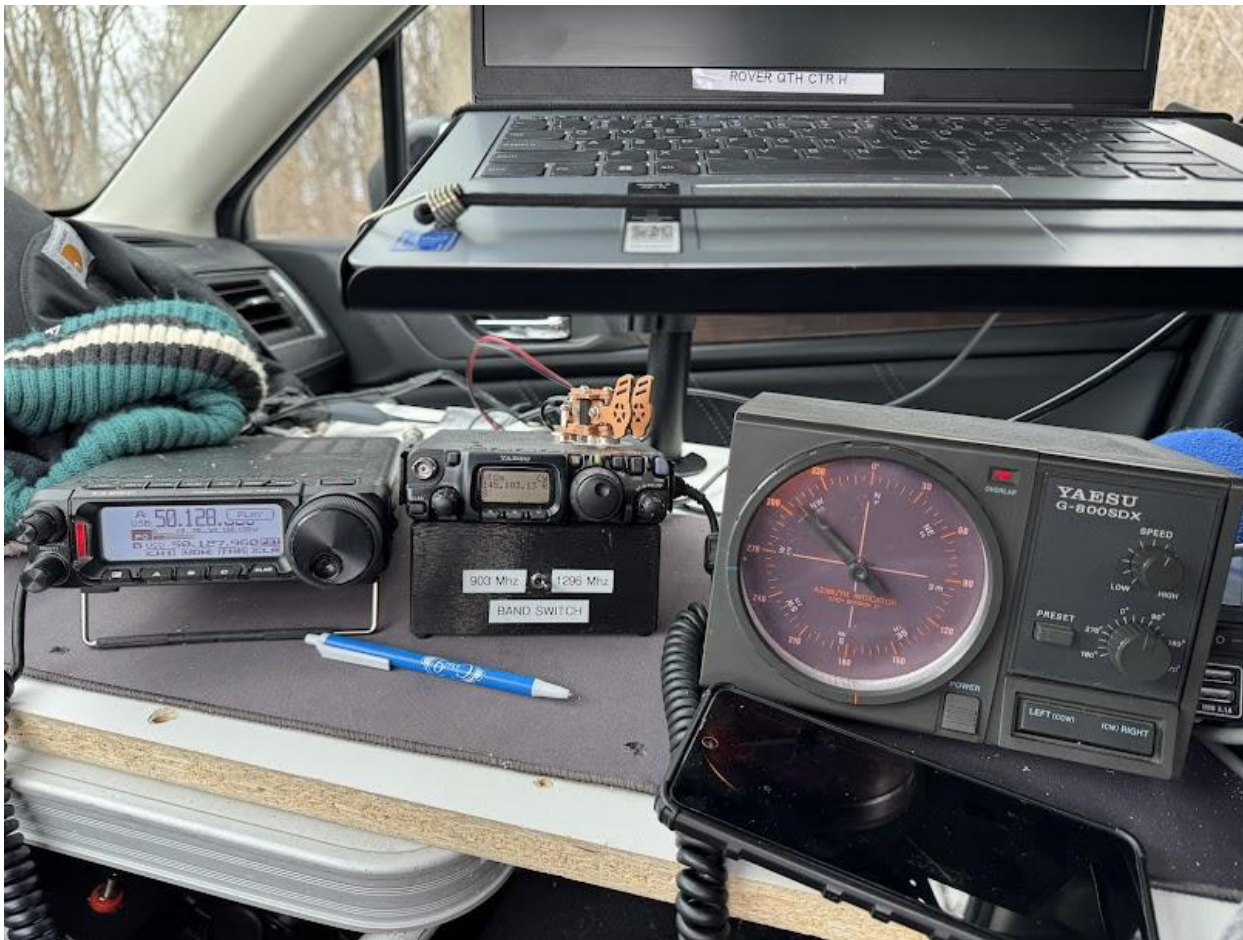
Rover Set up with the FT891, FT817, Rotor Control and Laptop Tray in the Passenger Seat
